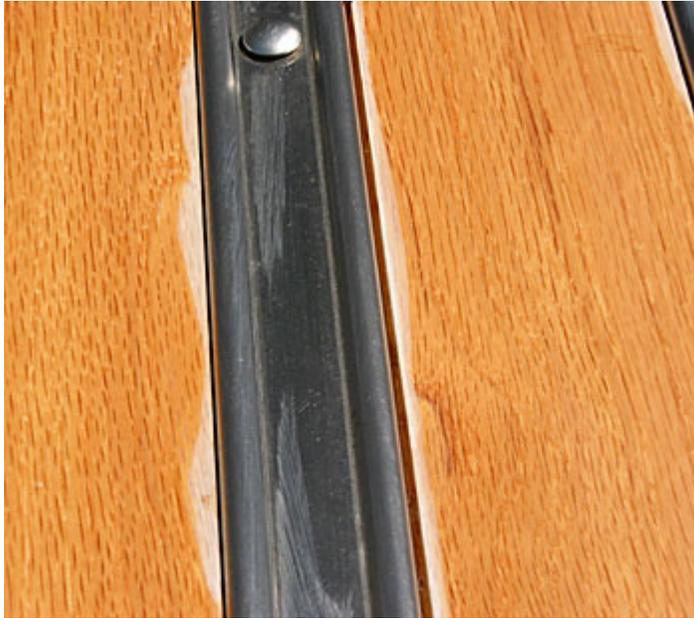
We noted in a previous update that the Glisten product, sample number 8, was failing. It is peeling away at the edges of several boards. This condition has worsened as shown in the photo.
