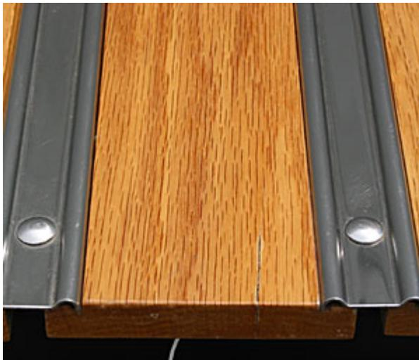
All the oak samples with natural finishes have some amount of failure. The best in these tests appear to be sample #6 and sample #1. Oak is especially susceptible to splitting on the ends and special care should be used to seal the ends as much as possible with the seal coat product. See Sample 6 left.
