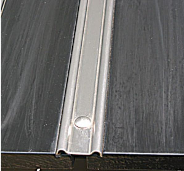
POR-15 Rust Preventative Paint appears to be an excellent primer/sealer and when used with a quality exterior paint should make a good choice for bed wood that is to be painted. See picture left.
