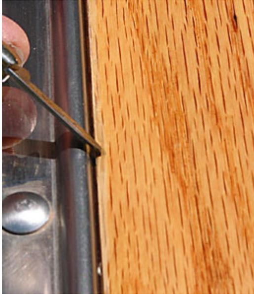
Sample number 10, a linseed oil seal coat with a Helmsman Spar Urethane topcoat, is now showing a small area of separation, see the photo. The wood is still protected under the varnish by the linseed oil but it will deteriorate soon without the urethane topcoat protection.
