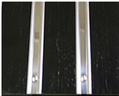
Behr black exterior latex enamel. This paint also developed small hairline cracks which indicates coating failure. The gloss seemed to be still good and no coating separation or peeling occurred. We will include a paint coating in the next tests. The specific brand and type have not been selected.
