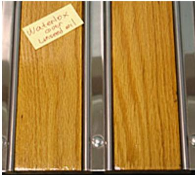
Using Linseed Oil to seal the wood before coating provided some benefit in preventing water damage, even when the coating film had small areas of failure. We hope to do more research here and find a way to evaluate this method of sealing the boards before coating.
