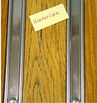
Waterlox The Waterlox used with the Waterlox sealer failed fairly early in the testing. It was not repaired. The Waterlox applied over dried linseed oil sealer lasted much better. It appeared to have a few minor cracks in the coating by the end of the test, but the linseed oil protected the underlying wood from extensive damage. These will be sanded and recoated for further testing.
