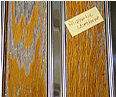
Aliphatic Urethane failed almost immediately. The manufacturer has suggested an alternative coating and application procedure. These will be included in the next coating tests.
