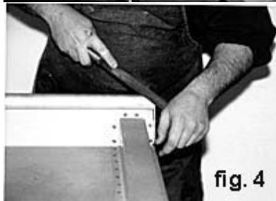
1. Make sure that the bed side panels are in good shape at the curl area and the top portion near the ends of the bed side. Straighten any bent areas on the top of the bed side and make sure that the curl is round.
