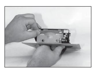
3. Insert the angle bracket between the upper two mounting points and the bracket welded to the adapter plate above the handle opening. The angle bracket should be positioned above the welded bracket.
