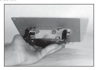
5. Attach the angle bracket to the welded bracket above the handle opening using two 8mm hex head screws and nuts. Tighten the bolts slightly to permit aligning the handle.
