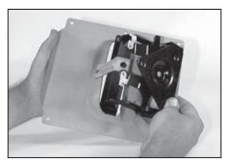
1. Hold the handle in the open position and while holding it open insert it into the opening from the back side. Be careful not to scratch the paint.
