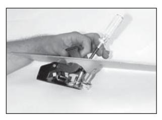
2. Use a cup washer and an 8mm hex head screw to attach the lower mounting point and the handle to the bracket on the adapter plate. Do not tighten the screw at this time.
