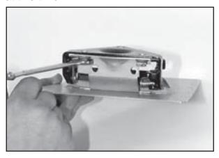
4. Use the two cup washers and 8mm hex head screws to attach the angle bracket to the upper two handle mounting points. Tighten the screws securely.
