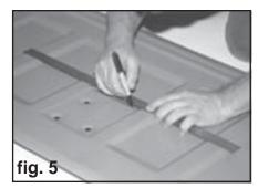
5. Using a suitable saw, grinder, or perhaps a plasma cutter, cut out the rectangular opening marked in #4 above. The curved surface makes this difficult and a small grinder may be needed to smooth the opening. The lower edge of the new opening is even with the lower edge of the original tailgate handle cutout on the other side of the tailgate. See figure 6.
