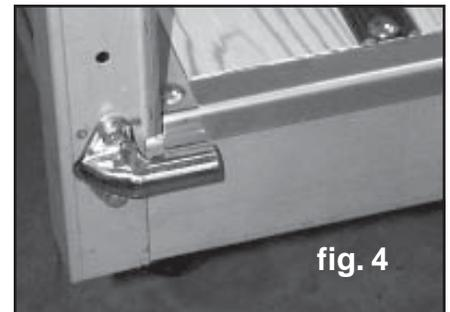
Install the right side hinge into the tailgate end. Place the tailgate onto the left hinge while bolting the right hinge to the right rear stake pocket. See figure 5. Use the same hardware on the right side including the 1/4" -20 x 5/8" hex bolt and the 1/4" -20 x 2-3/4" hex bolt, lock washer, and nut on the lower hole. Check that the tailgate does not bind when opening and closing it. Tighten all four bolts.
