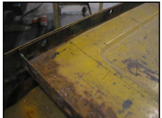
2. Mark and drill a hole where your line from the previous step crosses the curved area of the wheel house indentation. This will allow you to insert the jigsaw blade into this corner. Remember to drill the hole into the part being replaced below the line you marked. This hole will allow you to cut in either direction. You will make a cut following the shape of the wheel house opening through the bottom of the flange. Leave the curved section there so that there is something strong to weld to.
