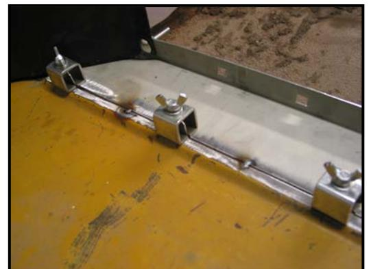
9. When you reach the wheel house with tack welds, you must remove the wheel house to tack weld behind it.
