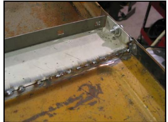
11. We need to re-create the two spot welds at the front panel flange that were drilled out. You will need to remove the paint around these holes also as shown. Clamp these panels together and weld through the holes that were drilled to remove the original panel. You may use an aluminum block or copper to back up the panel so that you do not burn through the repair panel with the plug weld.
