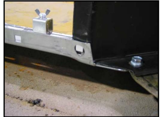
8. If the height measurements are good, tack weld the panel into place. Make small tack welds and space them apart far enough not to heat things up. We want to attach the two pieces together but not warp the panel with excessive heat.
