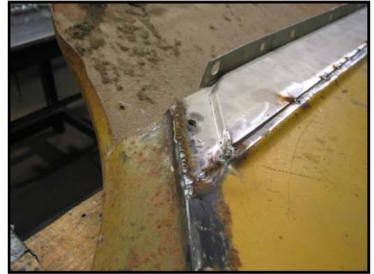
10. Continue tack welding until the entire seam has been filled. Don't forget the short vertical section at the front bedside flange. Move around while tack welding. If the panels are warm to the touch after a few welds, stop and take a break and let the panels cool.
