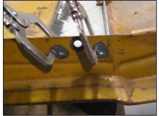
12. At this time, grind down the welds and check your progress.
