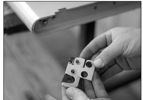
18. Attach each tailgate latch using two M6-1.0 x 30mm Phillips flat head screws. The u-shaped opening in the latch mechanism should line up closely to the notch in the tailgate end. The handle release mechanism protruding from the tailgate end should engage the latch. Use a thread locking compound on these screws.
