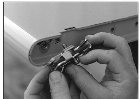
19. Place the check straps onto the bedside pins that are bolted to the inside of the bedside. In order to align the slots in the check straps fold the check straps in the opposite (upward) position while partially closing the tailgate.
