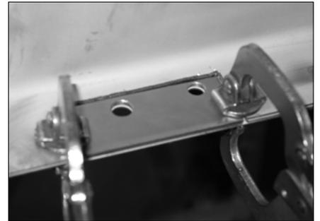
10. Tack-weld the patch into place from the outside of the bedside. Check to see that the patch has not shifted. Remove the template and tack weld from the other side. Do these steps to both bed sides.
