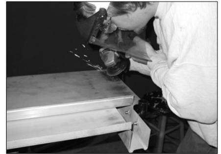
Note: The patch and the bedside should now appear to be the same metal and be smooth at the weld seam.
