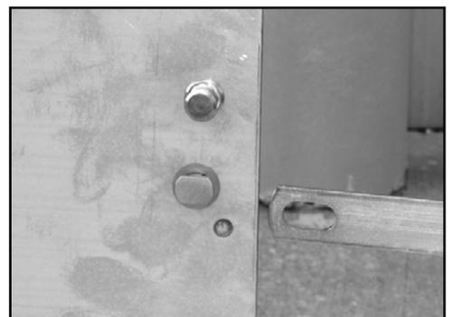
20. Once both check straps are placed on the pins, lower the tailgate to its full open position. Gently close the tailgate while watching the check straps. They should fold together towards the bedsides in a downward motion. Continue closing the tailgate. If any binding occurs, you may need to adjust a hinge up or down. If everything is good then close the tailgate against the strikers. Make sure the handle has been released to open the latches before doing this.
