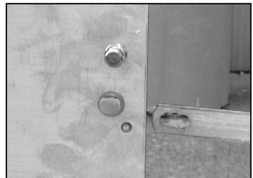
7. Once both check straps are placed on the pins, lower the tailgate to its full open position. Gently close the tailgate while watching the check straps. They should fold together towards the bedsides in a downward motion. Continue closing the tailgate. If any binding occurs, you may need to adjust a hinge up or down. If everything is good then close the tailgate against the strikers. Make sure the handle has been released to open the latches before doing this.
