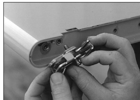
4. Install the check straps to each end of the tailgate using two 1/4-20 x 3/4 " button head torx screws with a T-25 torx driver.
