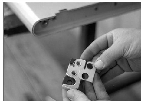
3. Attach each tailgate latch using two M6-1.0 x 30mm Phillips flat head screws. The u-shaped opening in the latch mechanism should line up closely to the notch in the tailgate end. The handle release mechanism protruding from the tailgate end should engage the latch. Use a thread locking compound on these screws.
