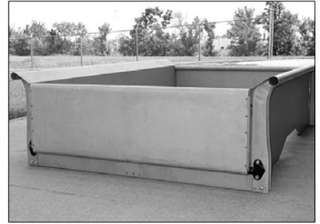
4. Remove one tailgate hinge so that you can remove the tailgate. Set the tailgate aside for now. Re-install the hinge at the scribed lines.
