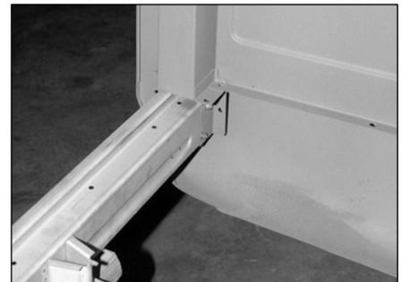
4. Bolt in place using (8) 5/16"-18 x 3/4" indented hex washer head bolts, (4) 5/16" lock washers, and (4) 5/16" nuts.
