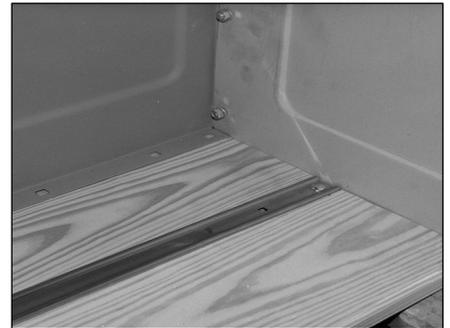
13. Install a 1/4"-20 x 1-1/4" carriage bolt through the rear bed strip to the rear cross sill and a 5/16"-18 x 1-1/2" carriage bolt through the front bed strip to the front bed panel lower flange. Minimize the gaps between the bed strip and the bed wood grooves and hand tighten bolts.
