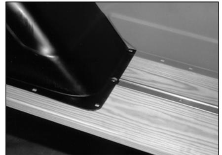
11. Place the short bed strips between these boards to ensure the right spacing. The bed strips will slide under the wheel well but on top of the boards. *If using MAR-K's custom bed strips with hidden fasteners, follow the instructions supplied with the bed strips for correct installation.*
