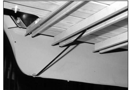
29. Install the wiring harness into the rear cross sill and up through the rear stake pockets on the bedsides. **(Hint:)** To pull the wiring up through the stake pockets, feed a metal wire down through the taillight opening. Attach to the taillight and back-up light wires and pull them up to the opening.
