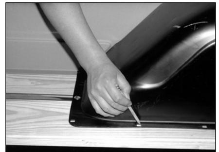
16. Replace the boards and install 5/16"-18 x 1-1/2" carriage bolts through the bedside lower flange and the wheel house lower flange through the boards. Leave the lock washers and nuts off of these bolts for now. Also reinstall the bolts at the end of the short strips with lock washers and nuts.
