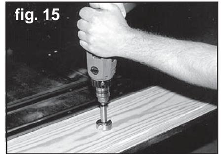
22. Using a 1-9/16" diameter Forstner bit, a drill press if available, or a hand drill, countersink each location approximately 1/8" to 5/32" deep. See figure 15.
