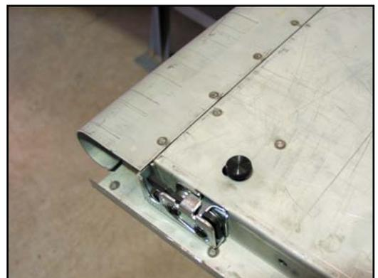
14. Bolt the link assemblies to each end of the tailgate. These are held in place by (2) ¼-20 x ¾" button head torx screws provided in the kit. Use a T27 torx driver to tighten these screws.
