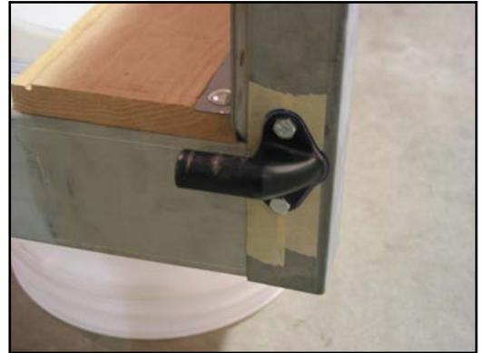
5. Slide the template provided onto the hinge far enough that the template can lay flat against the inside of the bedside. The outer edge of the template should be even with the outer edge of the bedside. Clamp the template in place. The template has been painted a dark color for the photo.
