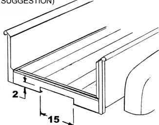
3. Temporarily clamp the pan side panels under the lower rear flanges of the bed sides so that the pan fits in position between the bedsides. The top of the pan should be tight against the rear sill. Check that the license box cut out allows clearance for the tag light socket and wiring.
