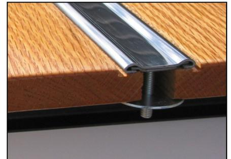
4. If installing the bed strips with hidden fasteners in a GM Fleetside box, there will be short strips that have an hole in one end of the strip. This end fits under the wheelhouse. A standard carriage bolt will fit into the wheelhouse flange and through the bed strip.
