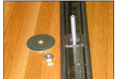
3. There may be a bed strip bolt in each space between cross sills that requires a 1-1/2" outside diameter washer with a 1/4" hole. This washer bridges the gap between the boards on the bottom and is placed on the bolt before installing the lock washer and nut.
