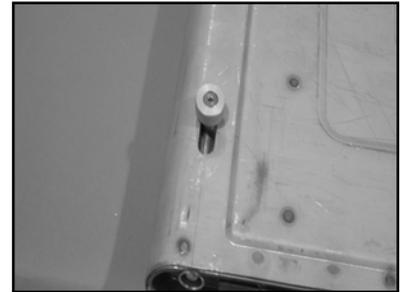
12. Remove the two bolts that hold the pivot bolt brackets to the upper portion of the bedsides. If yours are welded in, see the note below. It is not necessary to remove the brackets from the bedsides. Place the upper grommet brackets on top of these original brackets and re-install the bolts. Align the grommet brackets to the bedside outer profile and tighten these bolts. Due to the shape of these brackets, there is a left and right side and they will not fit if placed on the opposite bedside.
