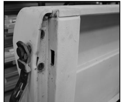
**Note:** If the brackets are welded to the bed side from the factory, You must drill and tap the original bracket to accept the grommet brackets. Place the grommet brackets into the upper corner of the bed sides. Mark the locations of the holes through the brackets. Drill and tap these locations to 5/16"-18. If you are not planning on using Mar-K's hidden link assemblies, you may also weld these grommet brackets in place.
