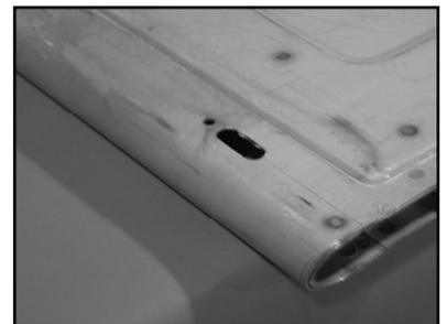
6. Disassemble the hidden latches by removing the aluminum knobs and the mounting screws. Slide the plungers and the springs out of the latch sleeves. Remove the #10-32 button-head screws from the latch sleeves.
