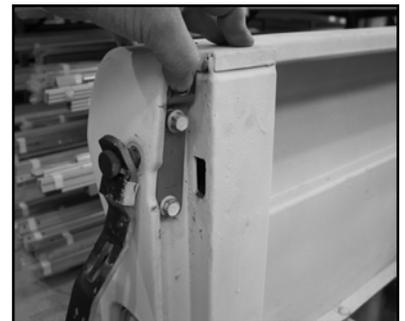
13. Once the latches are installed on both ends of the tailgate, re-install the tailgate on the truck. Make sure both latches are retracted and shut the tailgate. Hold the tailgate tight against the bedsides and release the latches by twisting the knobs. The latches have a pointed tip that will mark the bedsides for the rubber grommet to be installed.
