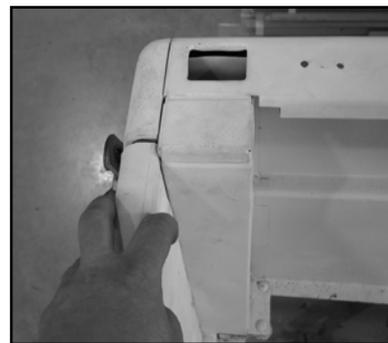
14. Lower the tailgate and support it in the open position. Each of the upper brackets should now have a mark from the latch plunger. Remove the brackets and drill a 5/8" diameter hole. Again, it is better to start with a small drill and work up to the 5/8" diameter to ensure a more uniform round hole. If you have access to a step drill, these tend to make perfectly round holes in sheet metal.
