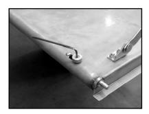
11. Test the movement of the plunger by sliding it back and fourth. Also pull the plunger all the way back and twist the knob to lock it in the retracted position. If the knob rubs on the tailgate or will not retract far enough to lock, you will need to enlarge the slotted hole in the tailgate with a file until full movement is obtained.
