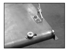
12. Place some masking tape onto the top rear corners of the bed sides as shown. Once the latches are installed on both ends of the tailgate, re-install the tailgate on the truck. Make sure both latches are retracted and shut the tailgate. Hold the tailgate tight against the bedsides and release the latches by twisting the knobs. The latches have a pointed tip that will mark the tape on the bedsides for the rubber grommet to be installed.
