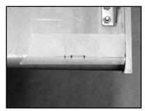
5. Using a small high speed cutting wheel, connect the two 3/8" diameter holes by cutting the metal out between them. This will create the slot that the knob on the latch will slide in.
