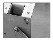
14. Insert the supplied rubber grommets into the bedside holes. Close the tailgate and release the latches into the grommets.
