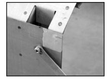
13. Lower the tailgate and support it in the open position. At each marked location on the bedsides, you need to drill a 5/8" diameter hole. Again, it is better to start with a small drill and work up to the 5/8" diameter to ensure a more uniform round hole. If you have access to a step drill, these tend to make perfectly round holes in sheet metal.
