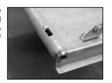
Install the spring on the plunger and slide it into the latch sleeve. A liberal amount of your favorite grease on the plunger is recommended before assembly.
