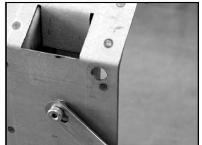
9. Insert the supplied rubber grommets into the bedside holes. Close the tailgate and release the latches into the grommets.
