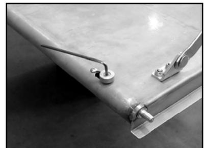
6. Test the movement of the plunger by sliding it back and fourth. Also pull the plunger all the way back and twist the knob to lock it in the retracted position. If the knob rubs on the tailgate or will not retract far enough to lock, you will need to enlarge the slotted hole in the tailgate with a file until full movement is obtained.
