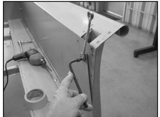
When repeating this procedure on the driver's side, the template will be positioned against the base of the bed side. Protect this area with a scrap piece of cardboard or wood. If you need further explanation of this procedure, go to [www.mar-k.com](http://www.mar-k.com) and click on the Installation information on the home page. Scroll down to "Other helpful information" and click on "Threaded insert Information".
