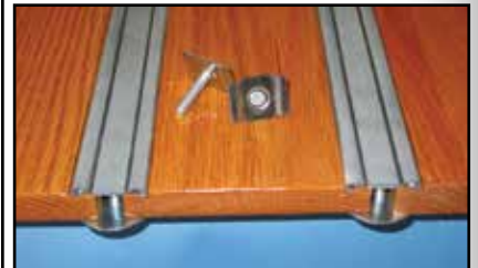
Steel must be painted to prevent rusting.
