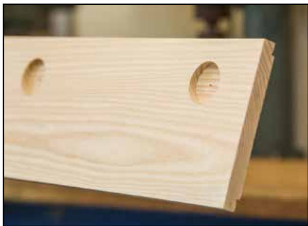
No Bolts Bed Wood: The bottom surface of the wood is drilled with a recessed clearance around the bolt head. The boards and strips rest on the cross sills as original, completely hiding the bed-to-frame and bed strip bolts.
