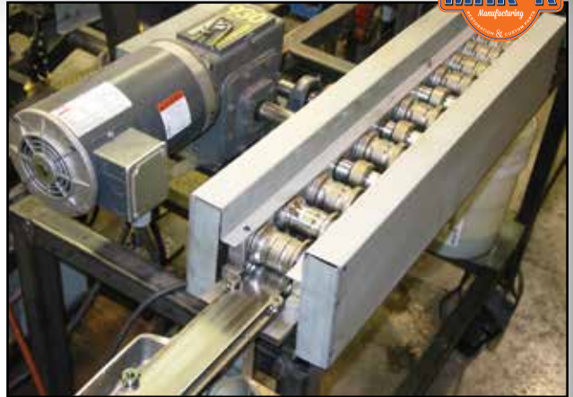
Polished stainless material is put in a roll former to make the bed strips with hidden fasteners.
