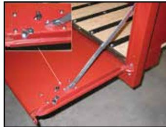
**MAR-K™** now makes a kit for installing the hidden rotary style latches and link assemblies into a stock Ford tailgate. Adapter panel is made of 16 gage electro-galvanized steel and link assemblies are available
