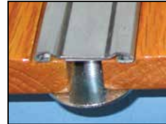
Polished stainless material is put in a roll former to make the bed strips with hidden fasteners.
