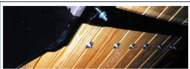
1972 GMC Stepside - William Thornton shows how the bed strip bolts fall between the wood boards and bolt underneath the wood. Where there is not a cross sill, the bolts are secured by flat washers.
