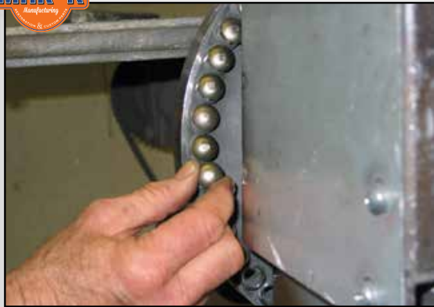
Unpolished stainless bolts are inserted into this special polishing machine to make the heads shine like chrome!
