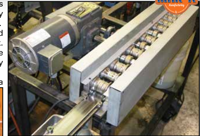
Polished stainless material is put in a roll former to make the bed strips with hidden fasteners.
