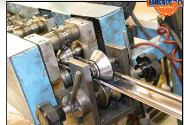
Polished stainless material goes through a special roll former to create the bend in angle strips.
