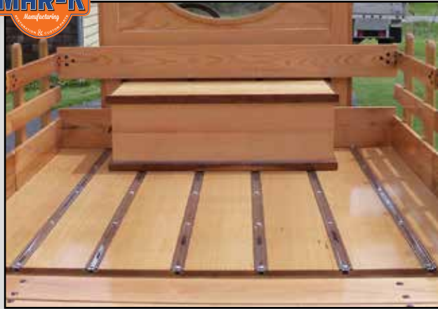
Custom made polished stainless bed strips complete the look of Larry Schuknecht's 1923 Model T Ford truck.
