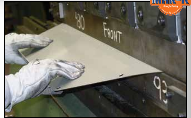
The top of MAR-K's™ Fleetside Repair Panels is embossed with an offset using this CNC press brake.
