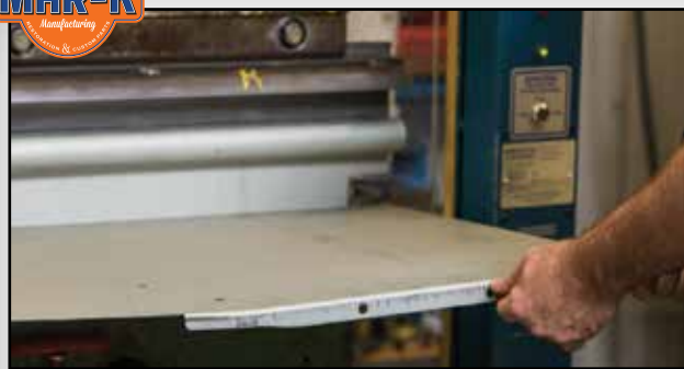
MAR-K™ bed side curls are formed in this tool in our bed side cell. It shapes the metal in a straight line and keeps it consistently strong and reliable.
